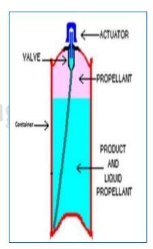
Aerosol products may be designed to expel their contents as a fine mist; a coarse, wet, or dry spray; a steady stream; or a stable or a fast-breaking foam. The physical form selected for a given aerosol is based on intended use.
