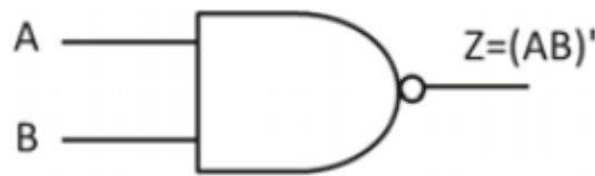
Fig. 3 AND gate with bubble at its output
