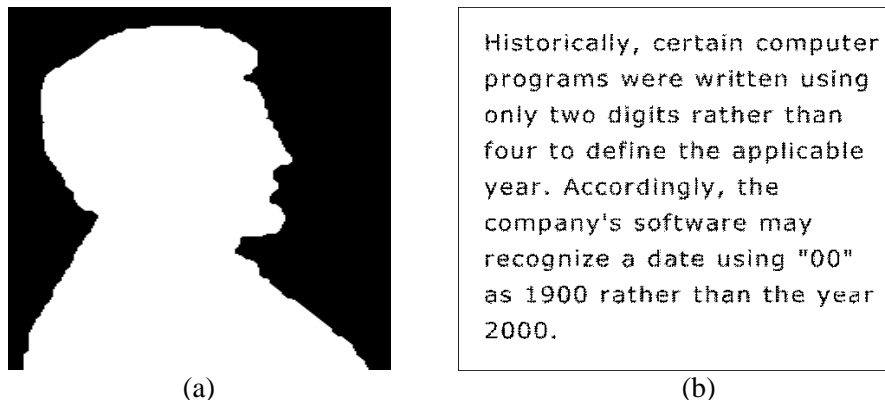
Figure 2.1 Binary images. (a) Object outline. (b) Page of text used in OCR application.
