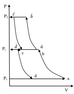
$$\frac{T_i}{T_1} = \left(\frac{P_i}{P_1}\right)^{(n-1)/n} \to T_i = (15 + 273)(3)^{(1.3-1)/1.3} = 371 \, K$$
