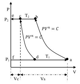
• The gas is then compressed according to the law  $[Pv^n = C]$  (in general) process (a-b). After that the delivery process begins from (b) to (c) as controlled by valves.
