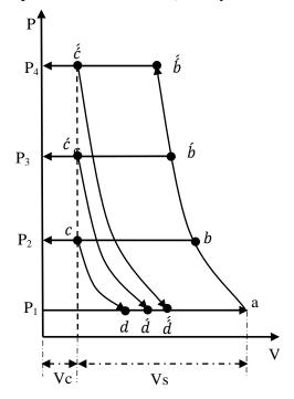
The indicator diagram for the two-stage machine is shown in the figure below. In this diagram it is assumed that the delivery process from the first or lowpressure stage and the induction process of second or high-pressure stage are at the same pressure.
