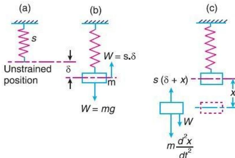
Fig. 2. Natural frequency of free longitudinal vibrations.
