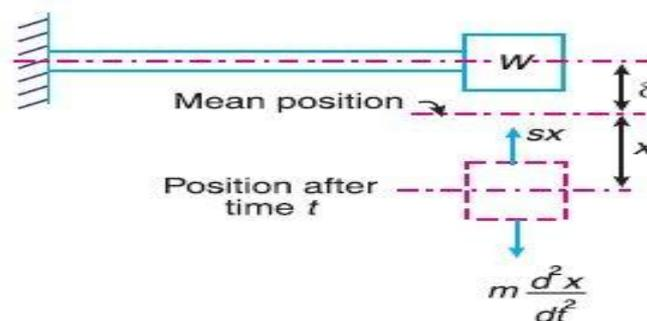
**Fig. 3.** Natural frequency of free transverse vibrations.
