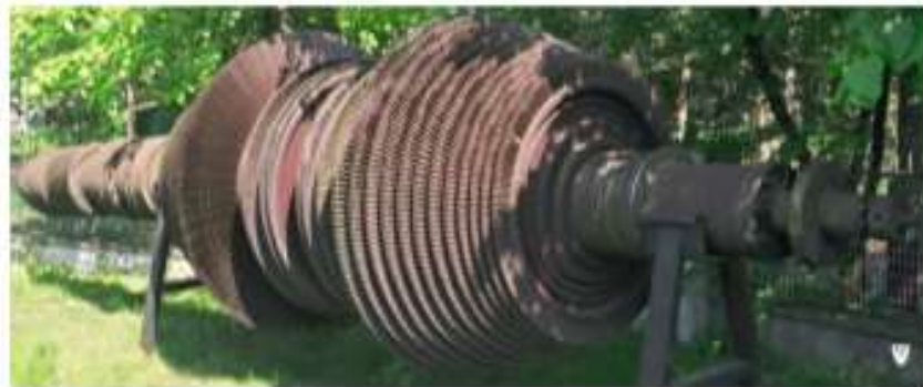
Figure 1: Parson turbine from the Polish destroyer ORP Wicher[1]
