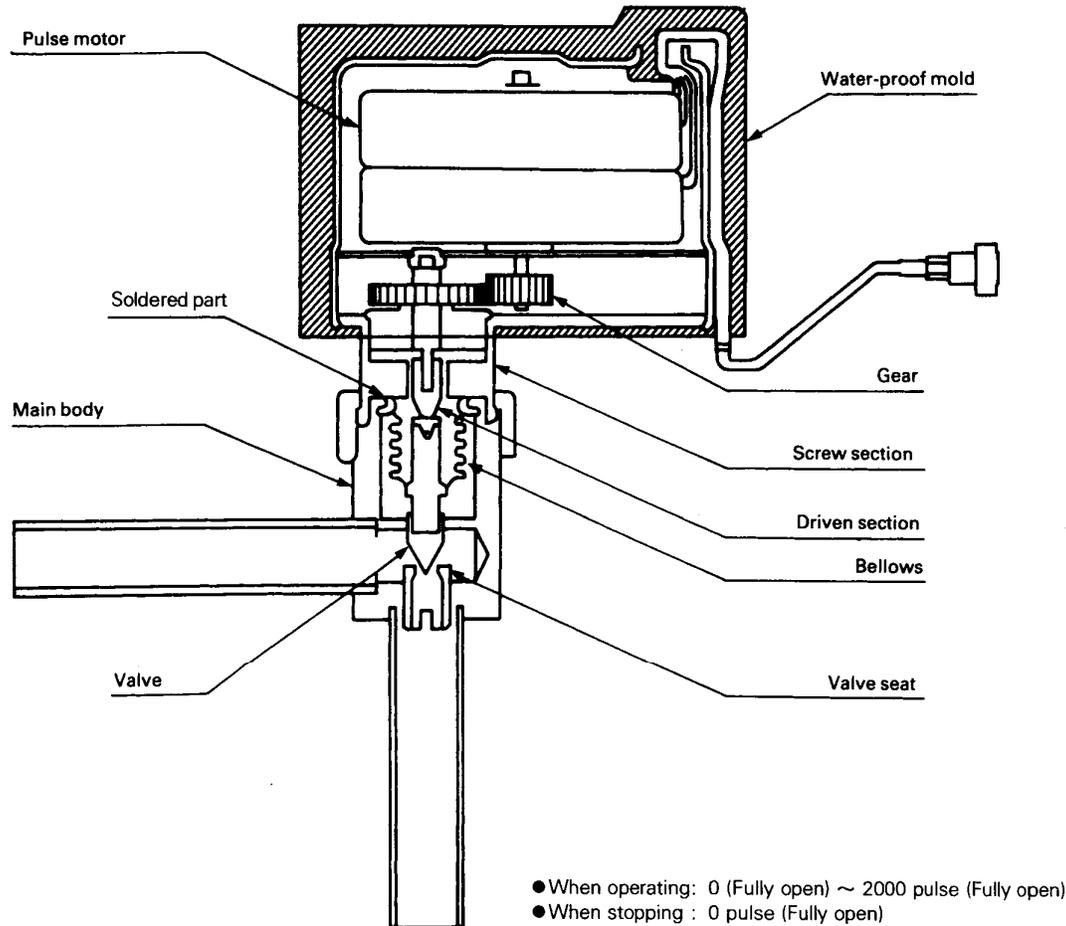
Structure of electronic expansion valve ... its main body and motor section
