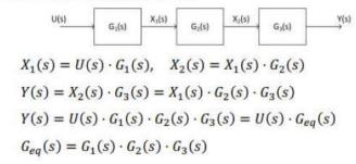
The equivalent transfer function of cascaded blocks is the product of the individual transfer functions
