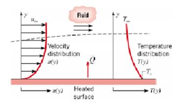
Coefficient of heat transfer by convection, h is not property of the fluid. It is a parameter which is determined experimentally. It is function of geometry of the surface, nature of fluid, properties and velocity of fluid. The following table gives typical coefficient of convection heat transfer.
