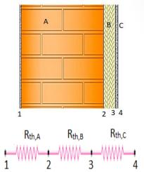
$$\dot{Q} = \frac{T_1 - T_4}{R_{th,A} + R_{th,B} + R_{th,C}} = \frac{1000 - 50}{0.136 + 0.833 + 0.0000125} = 980.38W$$
