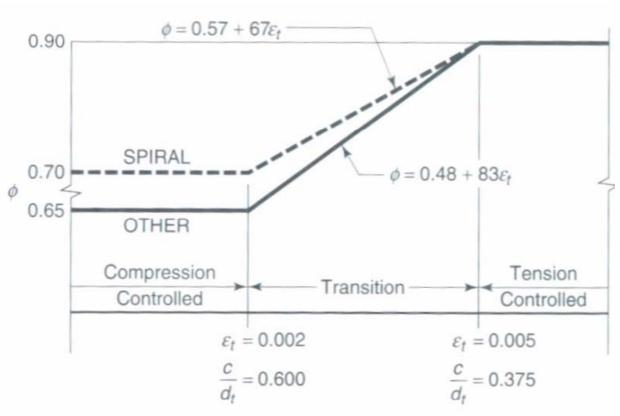
Interpolation on  $c/d_t$ : Spiral  $\phi = 0.37 + 0.20/(c/d_t)$ Other  $\phi = 0.23 + 0.25/(c/d_t)$
