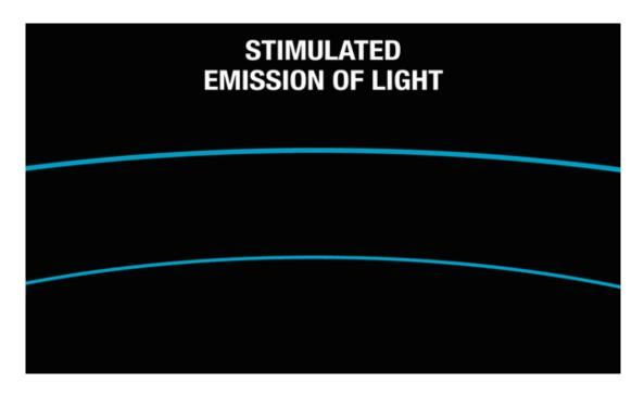
In a laser beam, the light waves are "coherent," meaning the beam of photons is moving in the same direction at the same wavelength. This is accomplished by sending the energized electrons through an optical "gain medium" such as a solid material like glass, or a gas.
