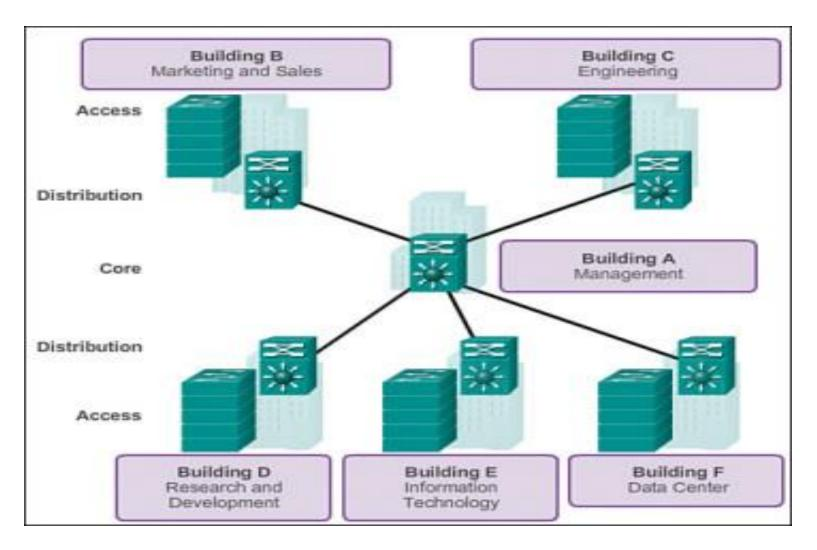
The actual manner in implementing the layers depends on the needs of the network to be designed. Each layer can be implemented in routers or switches. A particular layer can be omitted, but hierarchy should be maintained for optimum performance.
