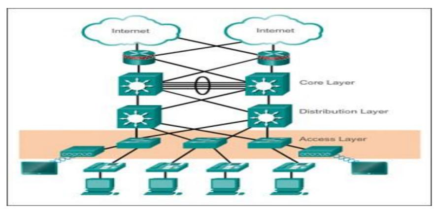
*the access layer* for a small business network generally incorporates Layer 2 switches and access points providing connectivity between workstations and servers.
