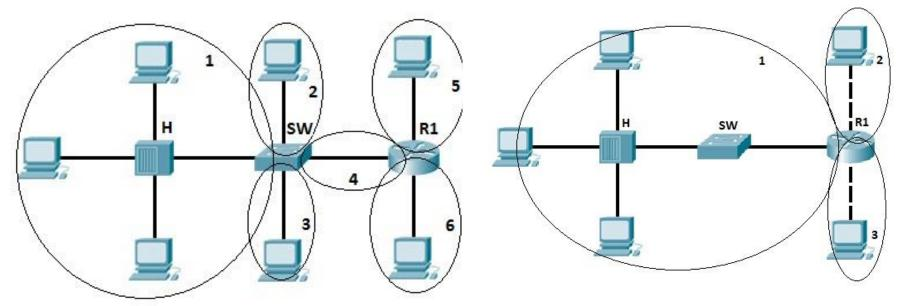
The packets collide and both devices must send the packets again, which reduces network efficiency. Collisions are often in a hub environment, because each port on a hub is in the same collision domain. By contrast, each port on a bridge, a switch or a router is in a separate collision domain.
