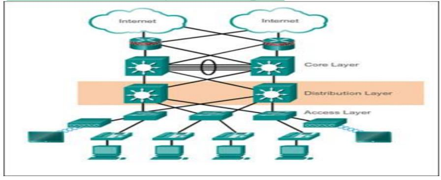
The *distribution layer* aggregates the data received from the access layer switches before it is transmitted to the core layer for routing to its final destination. In the distribution layer is the boundary between the Layer 2 domains and the Layer 3 routed network.
