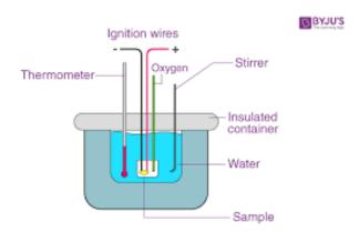
The heat capacity of the calorimeter is defined as: "the number of calories absorbed during the instant the calorimeter's temperature increases by one degree Celsius."
