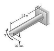
The solid shaft shown is made of a mild steel that is assumed to be elastoplastic with G=77.2 GPa and  $\tau_Y=145$  MPa. Determine the angle of twist caused by the application of a torque of magnitude (a)  $T=600~\mathrm{N\cdot m}$ , (b)  $T=1000~\mathrm{N\cdot m}$ .
