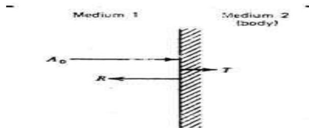
**Figure A sound wave of amplitude  $A_o$  incident upon the body.**
