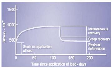
•Creep of concrete stored under such conditions (creep is simply taken as an increase in strain above the initial elastic strain) that no shrinkage or swelling takes place.
