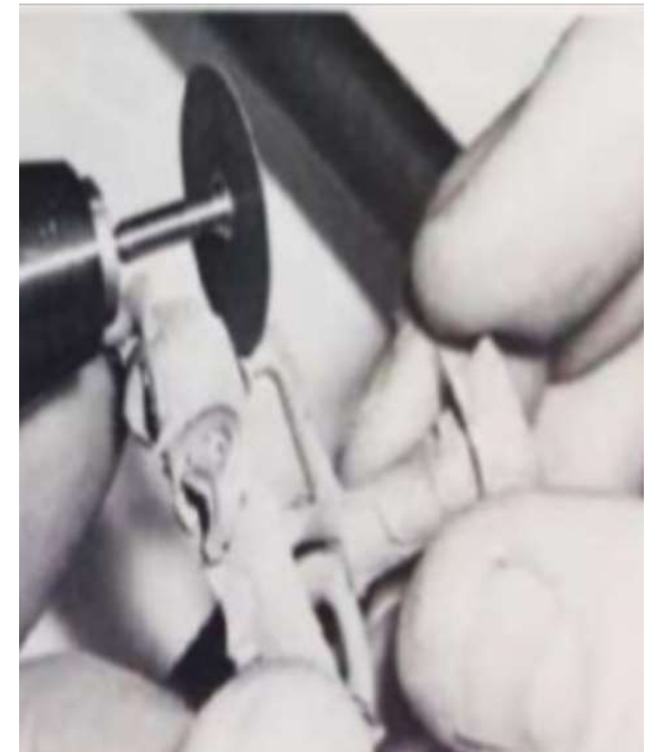
Figure 23: Left (abrasive disks), Right (the sprues are cut from the casting).
