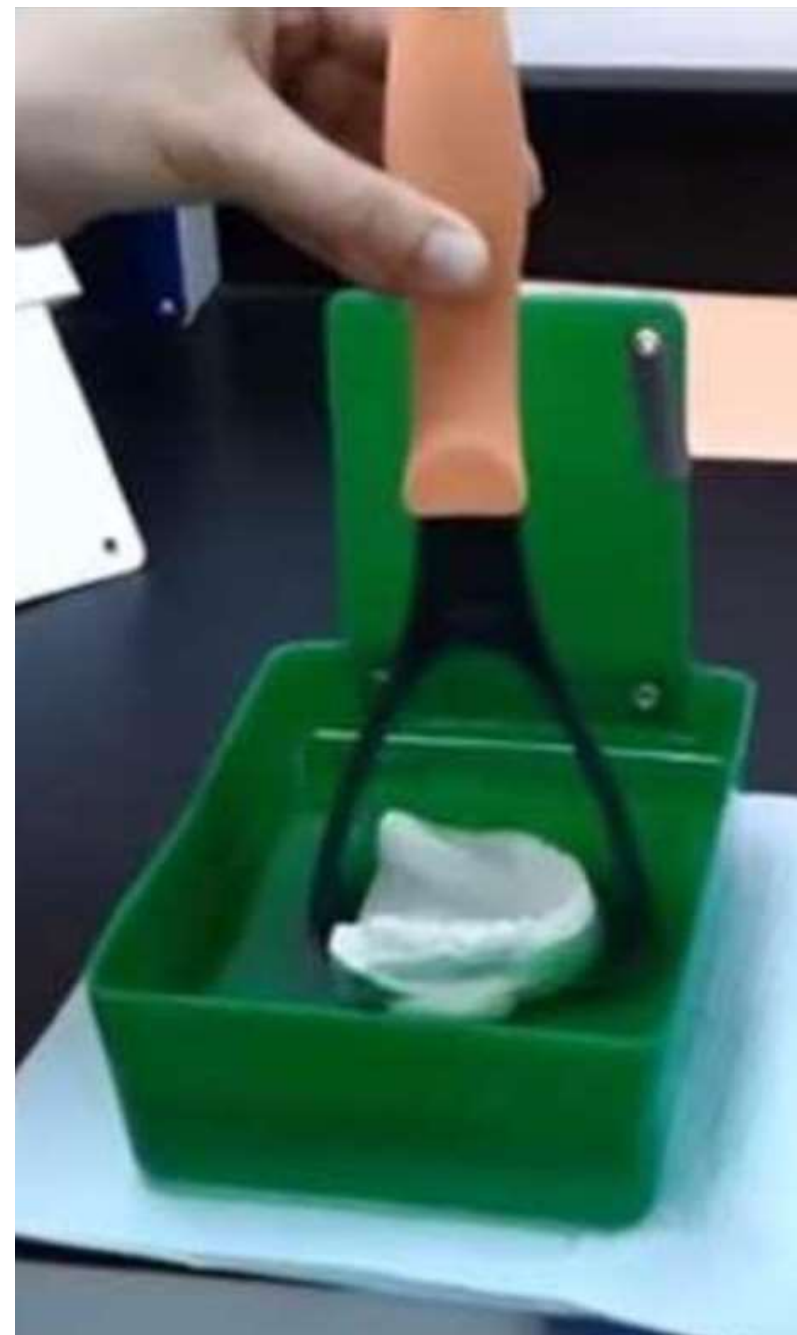
Figure 11: Left (refractory cast removed from dryness cabinet), Middle (the refractory cast is dipped in hot beeswax), Right (the refractory cast is allowed to dry).
