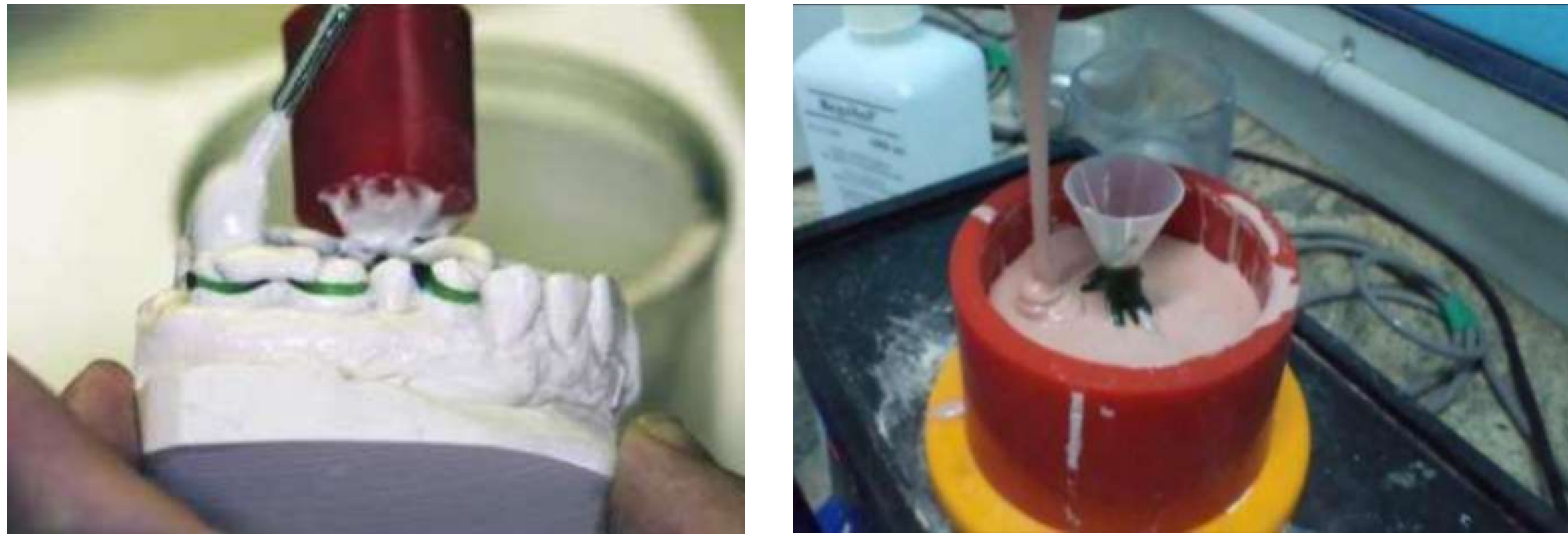
Figure 17: Left (sprued pattern on the refractory cast is poured with investment materials), Right (the refractory cast is completely poured with investment materials).
