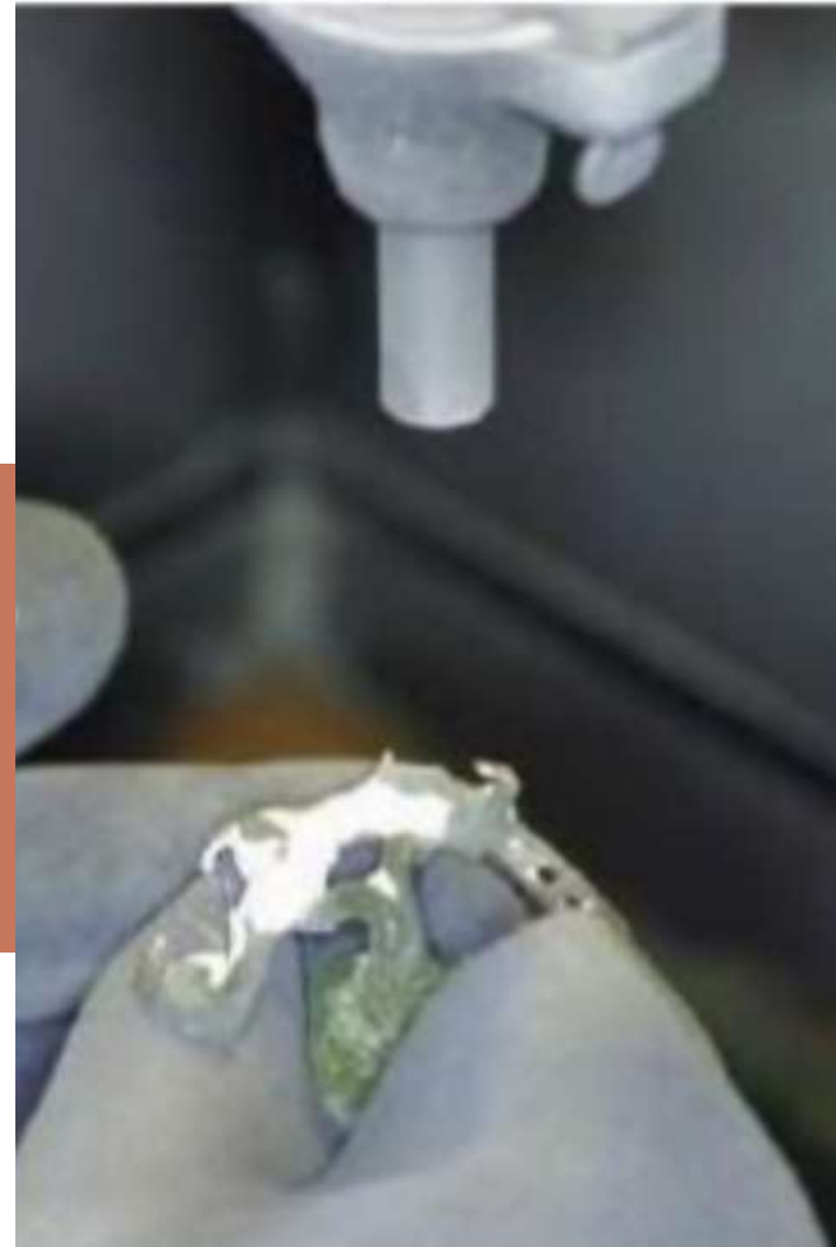
Figure 22: Left (airborne particle abrasion device), Middle (remaining investment is removed by airborne particle abrasion), Right (the casting after finishing abrasion).
