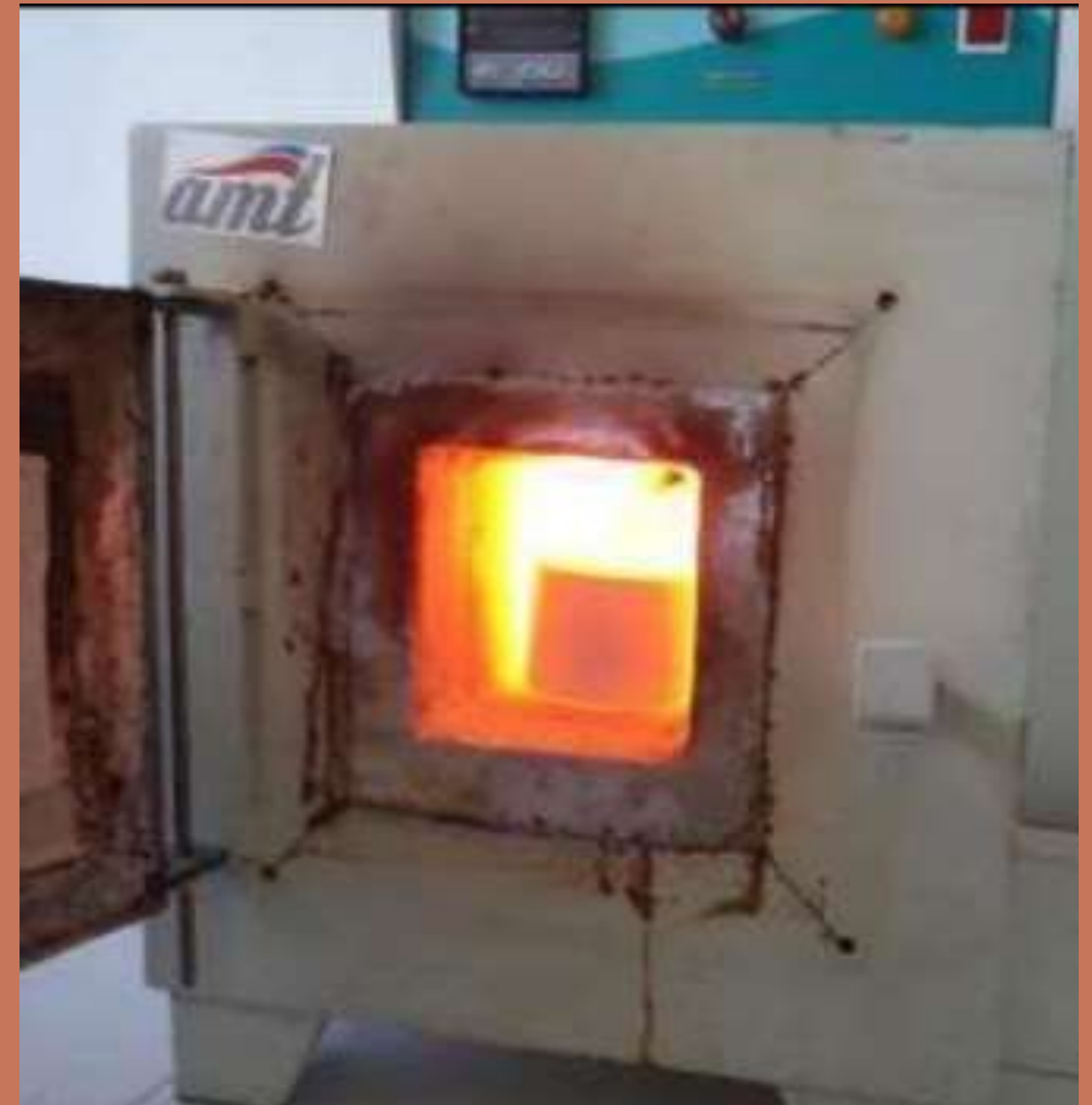
Figure 19: Mold is placed in the burnout oven for uniform heat penetration
