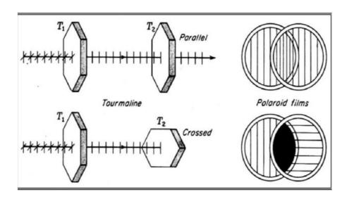
first crystal used is called the polarizer, which is The responsible for the formation of polarized light, and the second crystal that comes after the first is called an analyst, which is responsible for detecting whether the light will or not polarize completely or molecularly.
