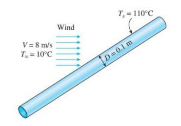
The Properties of air is evaluated at  $T_f = 60^o C$ Pr=0.7202, k=0.02808W/m.K,  $v=1.896x10^{-5}m^2/s$  $Re = \frac{D.u}{v} = \frac{0.1 \times 8}{1.896 \times 10^{-5}} = 4.226 \times 10^4$ C=0.027, m=0.805  $Nu = 0.027(Re)^{.805}(Pr)^{1/3}$  $= 0.027(4.226 \times 10^4)^{.805}(0.7202)^{1/3}$ = 128.15 $h = \frac{Nu.k}{d} = \frac{128.15 \times 0.02808}{0.1}$  $-=36W/m^2k$  $\dot{Q} = Ah(T_S - T_\infty) = (\pi dl)h(T_S - T_\infty) = (0.1\pi \times 1)36(110 - 10) =$ 1131*W*
