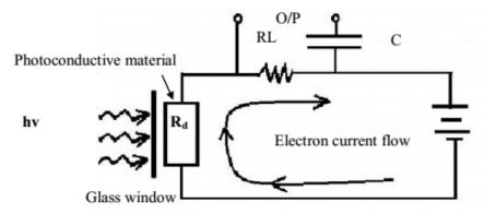
Photoconductive material decreases resistance as radiation applied.
