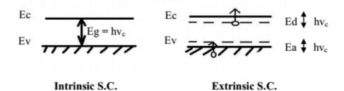
The smallest value of Eg at R.T. is  $\sim 0.15$  eV, enabling intrinsic s.c.s to be used for wavelengths up to 8  $\mu$ m.  $E_d$  and  $E_a$  can be arbitrarily small, which would enable extrinsic s.c.s to be used for arbitrary long  $\lambda s$ , except for a temperature limitation.
