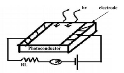
Flow which increases with the radiation intensity due to the release of more electrons in the photoconductor. The photoconductor is chosen such that its "dark" resistance is much larger than the load R<sub>L</sub>, and thus most of the bias voltage appears across the detector cell.
