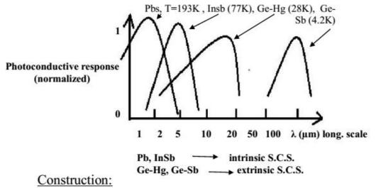
The photoconductive detector consists of a wafer of a s.c whose resistance decreases when it is illuminated by visible or IR light Mounted in an evacuated glass bulb.
