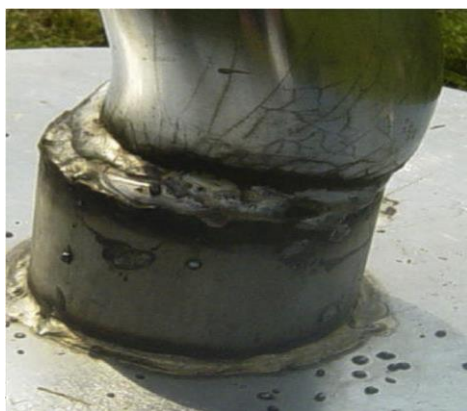
Stress corrosion cracking of austenitic stainless steel
