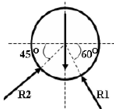
**Ex2:** Draw Free – body diagram for the 50 N sphere shown in fig.
