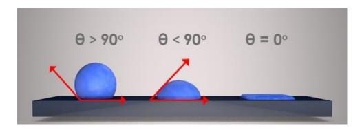
• A small contact angle indicates more adhesion is present because there is a large contact area between the adhesive and the substrate, resulting in a greater overall substrate surface energy and a high interactive force between the liquid and the substrate.
