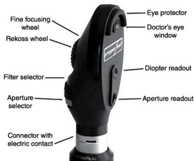
Figure 2 Various controls on a typical direct ophthalmoscope.
