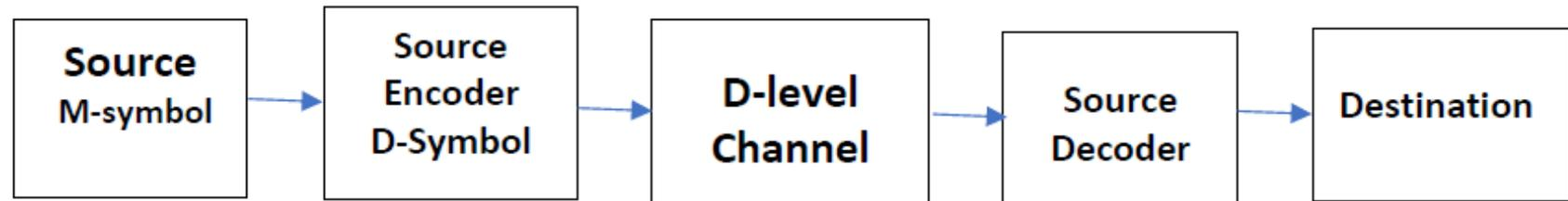
The function of the source encoder is to map each code symbol into corresponding coded word with D-level digits. The mapping should be unique or one-to-one mapping. In the case of binary code ( $D=2$ ) the source encoder output is connected to 2-level channel or binary channel (as in BSC). The source decoder will map the coded alphabet symbols into source symbols  $x_i$ .
