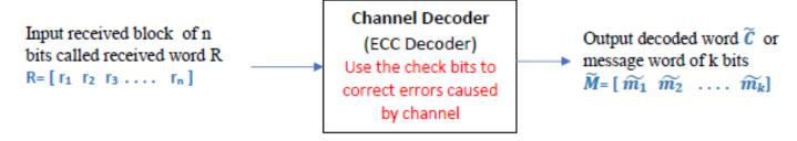
In above model  $m_i$ ,  $c_i$ ,  $r_i$  and  $\widetilde{m_i}$  are binary values "0" or "1".
