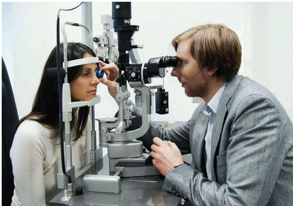
Figure .3 Slit lamp in use. Source: Mr. PFrankoZeitz, https://commons.wikimedia.org/wiki/File:Slit_lamp_examination.jpg .
