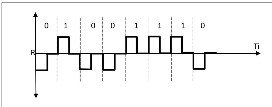
The main *disadvantage* of RZ encoding is that it requires two signal changes to encode one bit and therefore requires more bandwidth.
