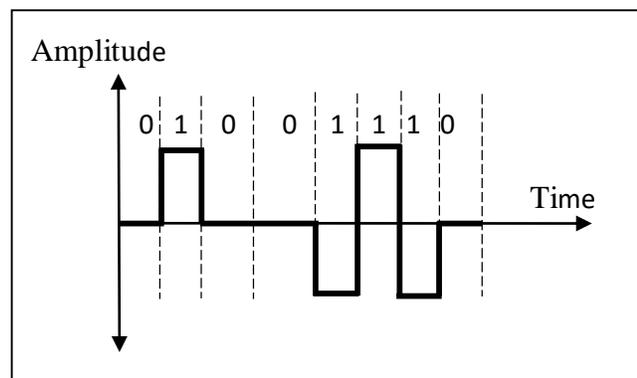
The other bipolar types have been developed to solve the problem of synchronizing sequential 0's.
