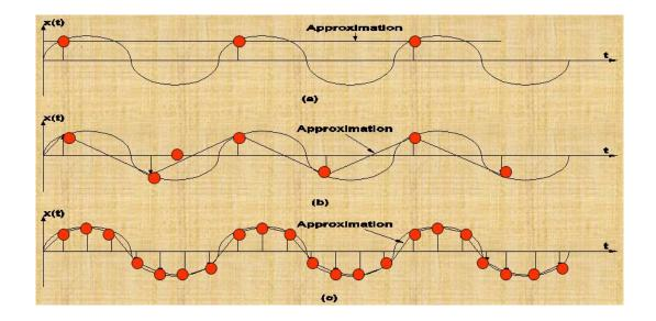
**Overall Better Accuracy:** Increasing both the sampling rate and the resolution you can obtain better accuracy in your AD signals.
