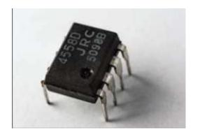
Figure 1 shows a typical op amp package.
