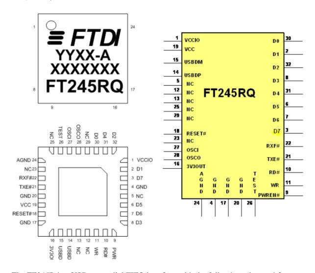
The FT245R is a USB to parallel FIFO interface with the following advanced features:
