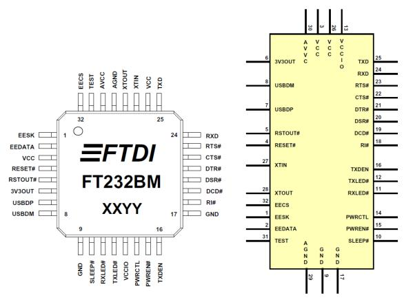
The FT232BM is a USB to serial UART interface with the following advanced features:
