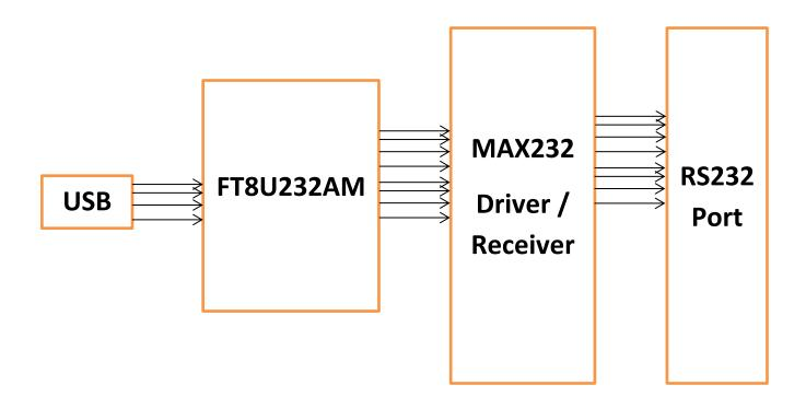
We will separate the design into two parts: the first part is the connections between USB and FT232BM and the second part is the connections between FT232BM and RS232 through MAX232.
