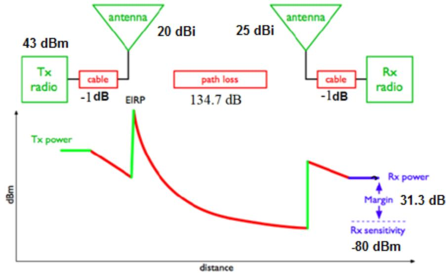
Q8/ Calculate the link budget for the 10km transmitting distance of 20w power that is applied to the transmitter with antenna gain of 20dBi and transmitter sensitivity of -85 dBm. The receiver (Rx = 18w) is connected to an antenna with 25dBi gain and a receive sensitivity of -80 dBm. The cables in both systems are short, with a loss of 1 dB at each side at the 13 GHz frequency of operation.
