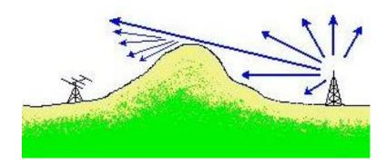
The radio wave changes in amplitude and phase and penetrates the shadow zone, deviating from a straight line path.
