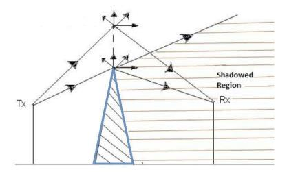
• Knife-edge diffraction model is one of the simplest diffraction model to estimate the diffraction loss. It considers the object like hill or mountain as a knife edge sharp object.
