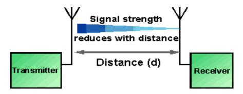
The **path loss** represents signal attenuation as a positive quantity measured in dB, is defined as the difference between the transmitted power and the received power.
