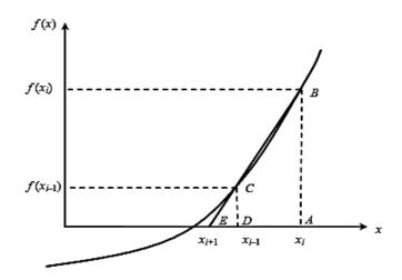
Example 1/ Find the root of the function by Secant method
