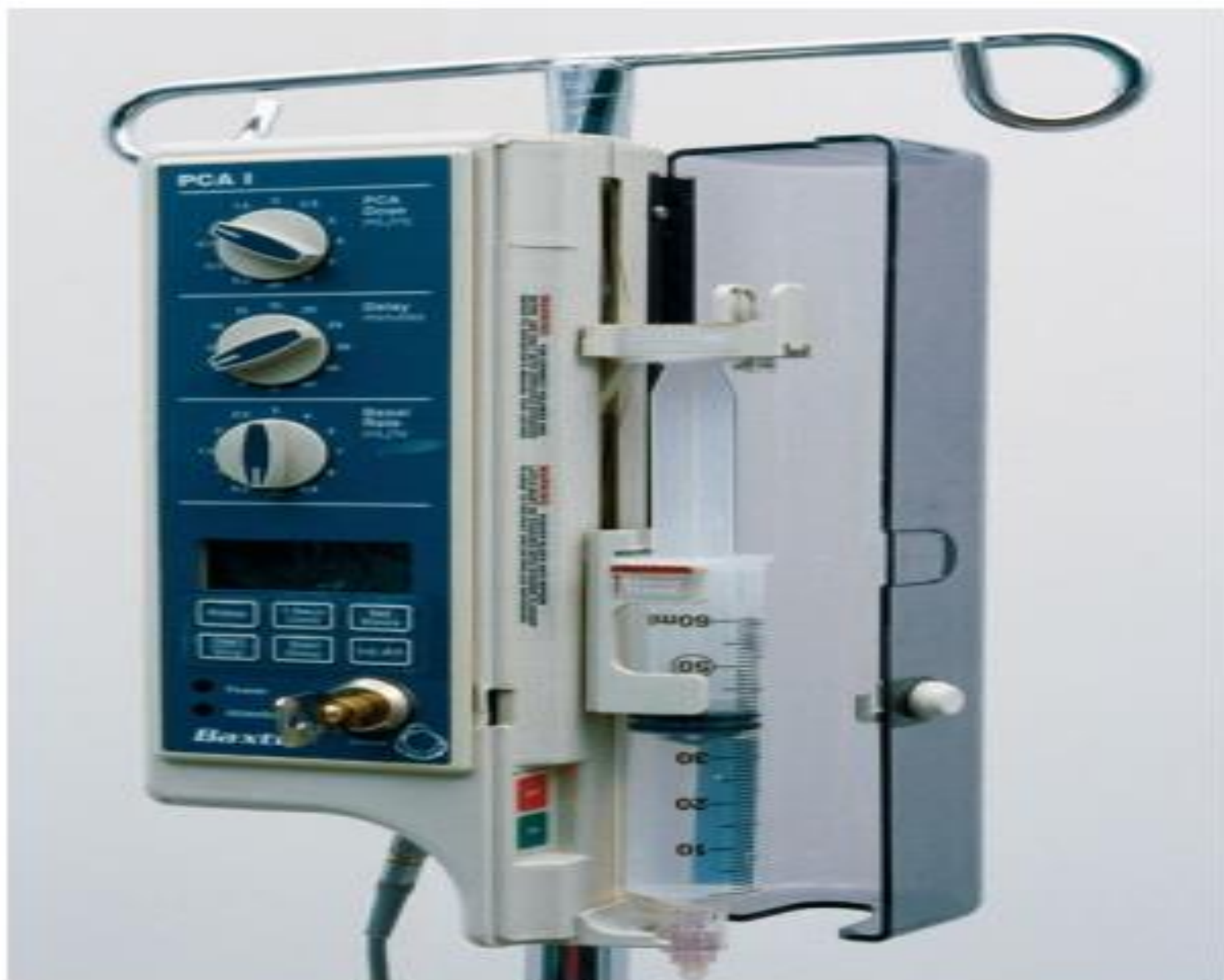
Figure 35–47 ■ Syringe pump or mini-infuser for administration of IV medications.
