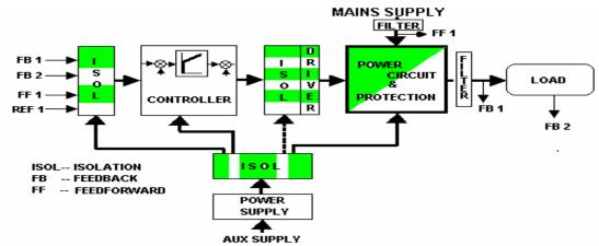
Fig. 1.1 The block diagram of a typical Power Electronic converter
