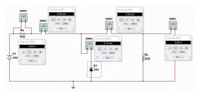
**Ex2:** A 5.0V stabilized power supply is required to be produced from a 12V DC power supply input source. The maximum power rating Pz of the Zener diode is 2W. Using the Zener regulator circuit above calculate:
