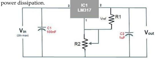
LM317 Voltage Regulator Circuit
