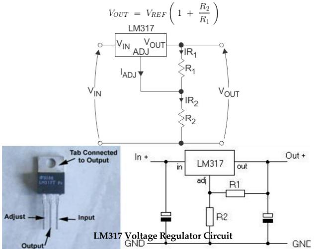
The three terminals are input pin, output pin and adjustment pin. The LM317 circuit is shown in the below figure is a typical configuration of the LM317 voltage regulator circuit diagram including the decoupling capacitors. This LM317 circuit is capable to provide variable <u>DC power supply</u> with output of 1A and can be adjusted up to 30V. The circuit consists of a low-side resistor and high-side resistor connected in series
