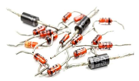
The values of the individual Zener diodes can be chosen to suit the application while the silicon diode will always drop about 0.6 - 0.7V in
