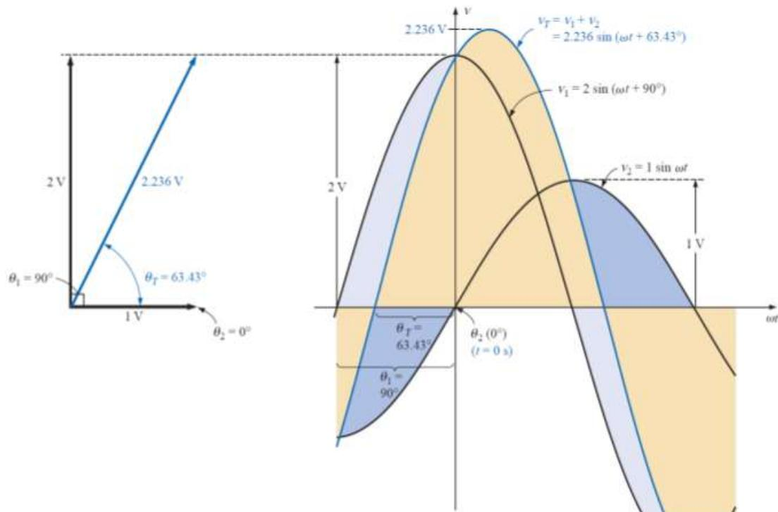
$$e = V_m \sin(\omega t + \theta) \Rightarrow e = \frac{V_m}{\sqrt{2}} \angle \theta = 0.707 V_m \angle \theta$$
