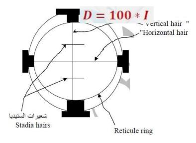
Where D is the distance from instrument to rod, and I is the stadia interval (upper minus lower rod reading)
