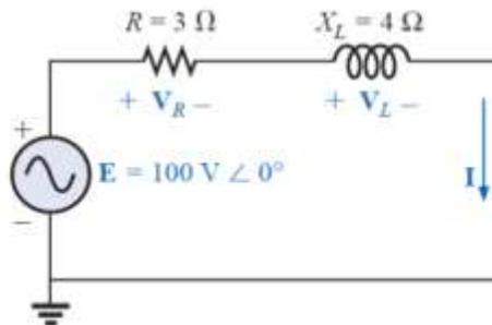
$$\mathbf{Z}_T = \mathbf{Z}_1 + \mathbf{Z}_2 = 3 \Omega \angle 0^\circ + 4 \Omega \angle 90^\circ = 3 \Omega + j4 \Omega$$
