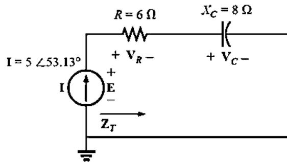
$$\mathbf{Z}_T = \mathbf{Z}_1 + \mathbf{Z}_2 = 6 \Omega \angle 0^\circ + 8 \Omega \angle -90^\circ = 6 \Omega - j8 \Omega$$
