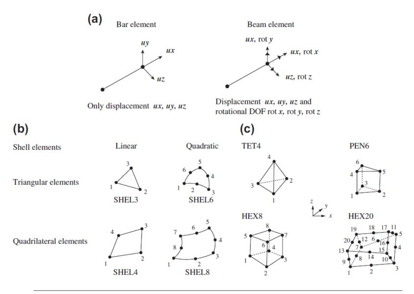
Typical finite element types: (a) bars and beams; (b) 2D shell elements; (c) 3D solid elements.
