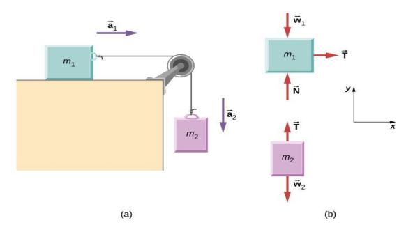
We draw a free-body diagram for each mass separately, as shown in Figure. Then we analyze each one to find the required unknowns. The forces on block 1 are the gravitational force, the contact force of the surface, and the tension in the string. Block 2 is subjected to the gravitational force and the string tension. Newton's second law applies to each, so we write two vector equations:
