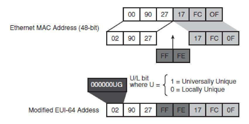
The seventh bit in an IPv6 interface identifier is referred to as the Universal/Local (U/L) bit. This bit identifies whether this interface identifier is locally unique on the link or whether it is universally unique.
