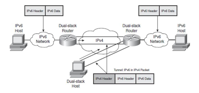
By using overlay tunnels, isolated IPv6 networks can communicate without having to upgrade the IPv4 infrastructure between them. Both routers and hosts can use tunneling. The following different techniques are available for establishing a tunnel:
