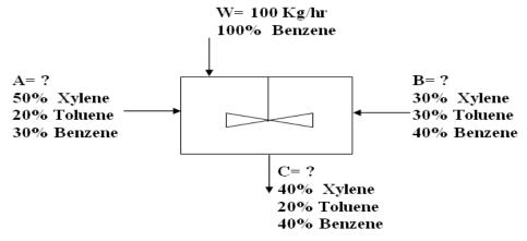
Solution: By making component material balance on each component within the mixer you can reach to a system of three equations which can be solve by using the command solve to find the unknowns A, B, C.
