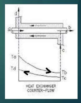
Solution: Counter flow heat exchanger is used to cool oil of mass flow rate
