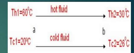
Counter flow heat exchanger: The log mean temperature difference is calculated for the counter flow as that in the parallel flow heat exchanger but the direction is be oposit as below
