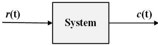
Fig. (5-2): Block diagram of a general control system.
