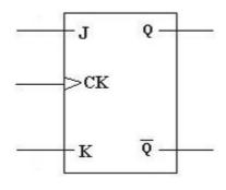
A circuit symbol for a Positive edge triggered JK flip-flop, where > is the clock input, J and K are data inputs, Q is the stored data output, and Q' is the inverse of Q The characteristic equation of the JK flip-flop is:
