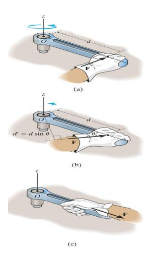
In addition to the tendency to move a body in the direction of its application, a force can also tend to rotate a body about an axis. The axis may be any line which neither intersects nor is parallel to the line of action of the force. This rotational tendency is known as the moment M of the force. Moment is also referred to as torque.
